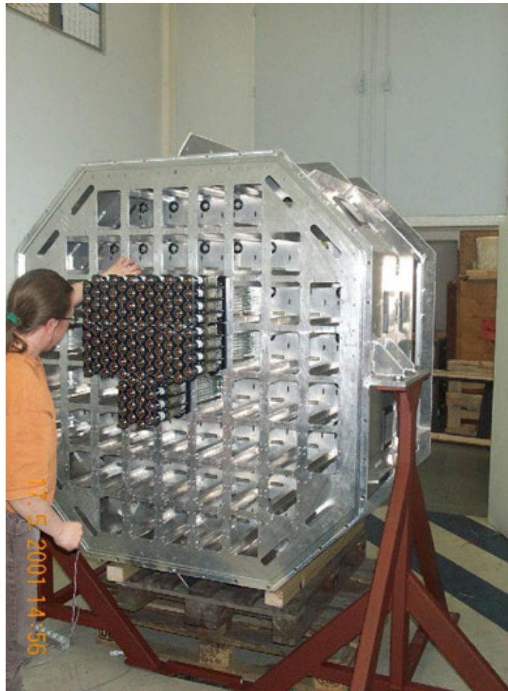
Figure 2.26: The HESS camera in the process of being filled with photomultipliers.
