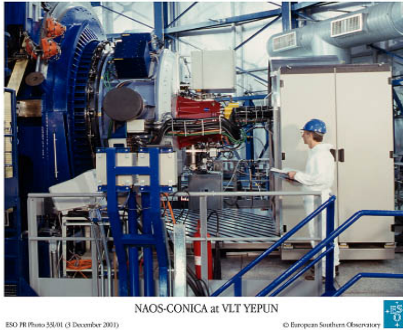
Figure 2.9. NAOS-CONICA at the VLT. From left to right: the telescope adapter (dark blue), NAOS (light blue), and the CONICA cryostat (red). The control electronics is located in the white cabinet.
